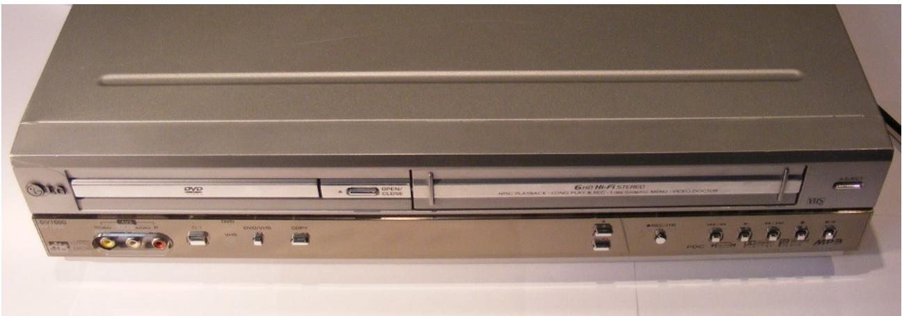
The yellow, white & red inputs on the bottom left look like a good fit, don't they? Actually, they're an input for a camcorder, and we need an output. Never connect our leads to the front of a VCR.
