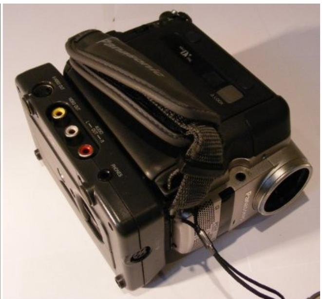
NOTE: A Camcorder with a MiniDV output will give better results if connected by a Firewire cable to a Firewire port on your PC. If you capture using an analogue device you are losing some quality.
